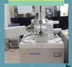
FESEM is to observe small structures (as small as 1 nanometer until one billion of a millimeter) on the surface of cells and material.
